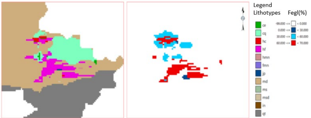
Figure 11-27 — Visual comparison of the geological model (left) with the estimated global iron grades (right) for bench 622.5
